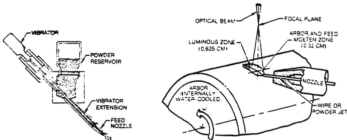
Figure 8: LAYERGLAZE™ Powder Method
