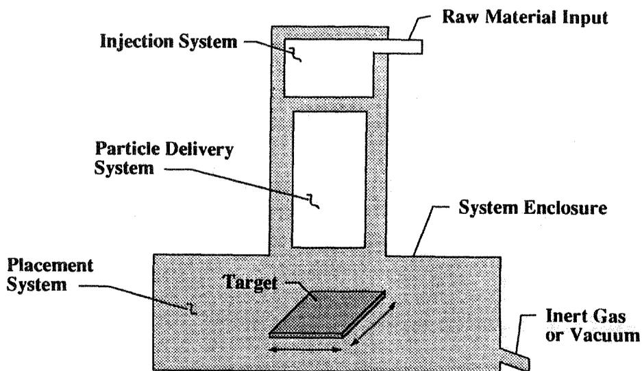
Figure 7: Ballistic Particle Manufacturing (BPM)
