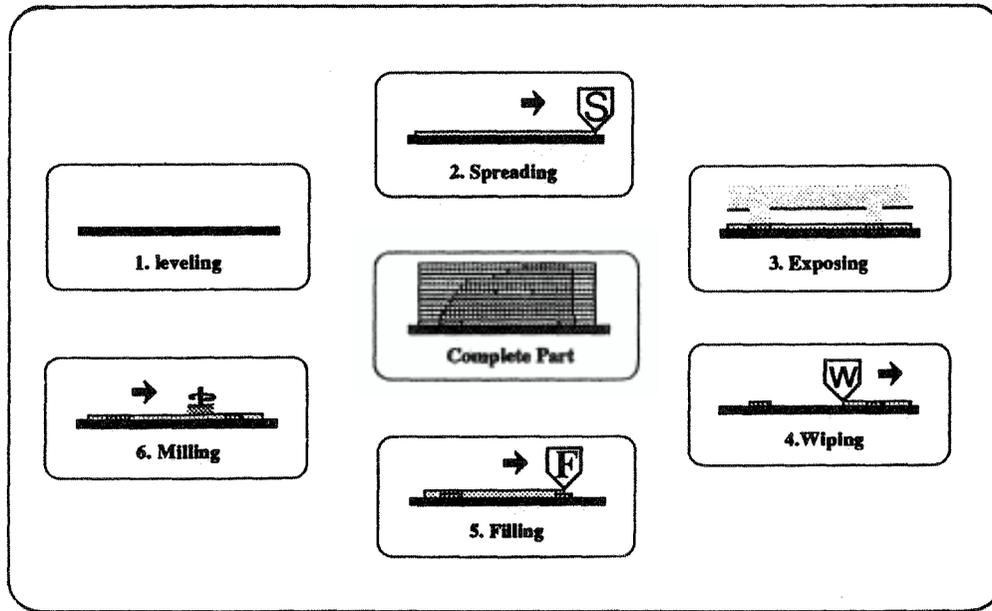
Figure 3: Cubital Instant Slice Curing Solder System
