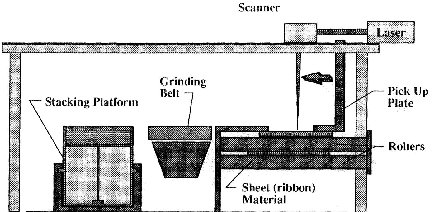
Figure 6: Laminated Object Manufacturing (LOM)
