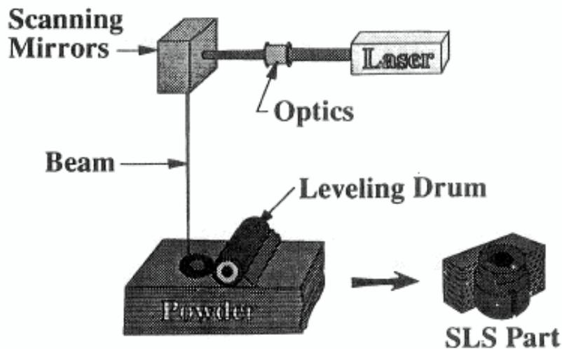
Figure 5: Selective Laser Sintering (SLS)
