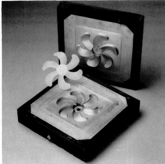
**Figure 1: Zinc Molding die for a fan blade**
