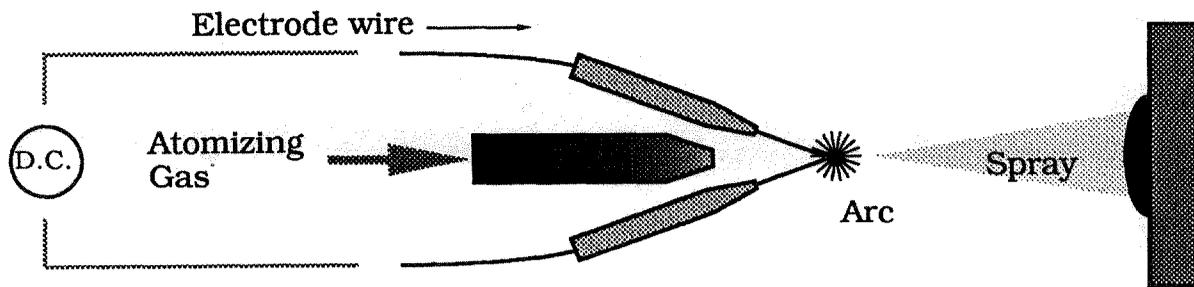
**Figure 2: Schematic of Arc-Spray System.**
