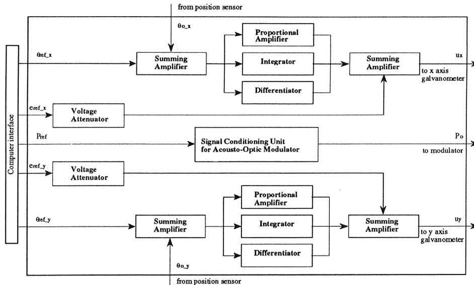
**Figure 6** Block diagram of dual channel analog controller
