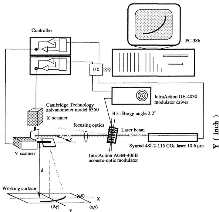
fig.1 The scanner control system
