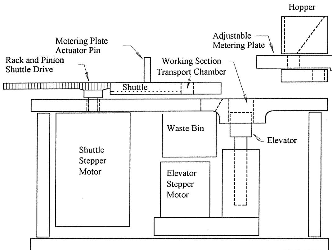
Figure 1: Powder handling system.
