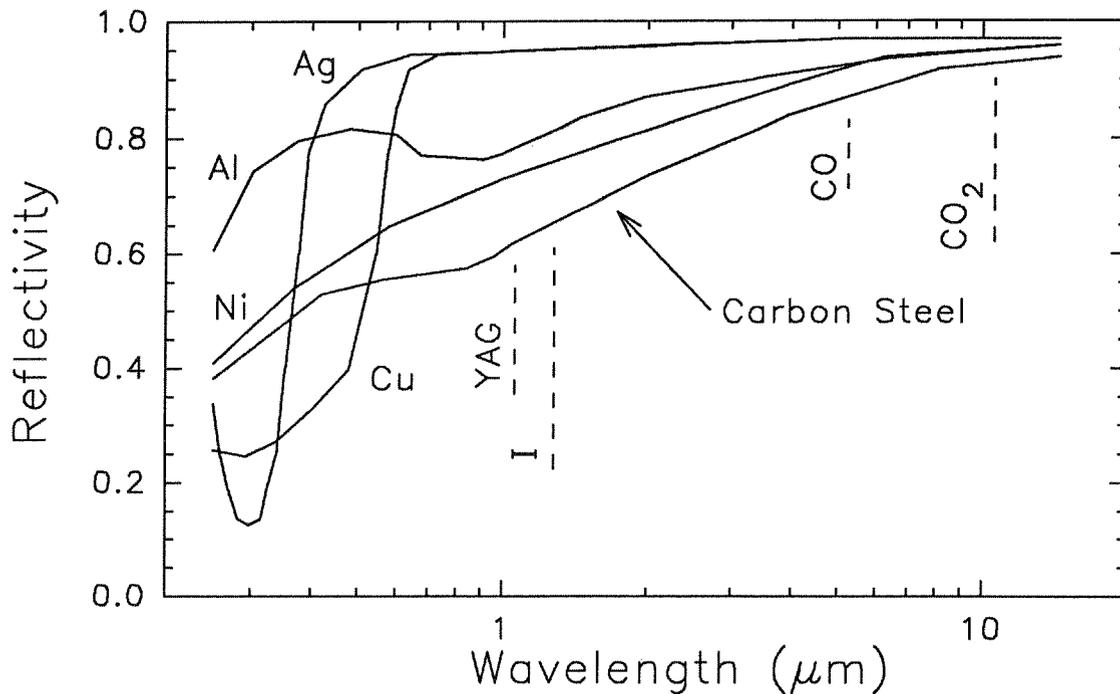
Figure 2: Wavelength dependence of reflectivity for various metals.
