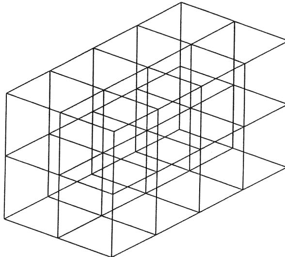
**Figure 1** Finite element model of right, rectangular prism.
