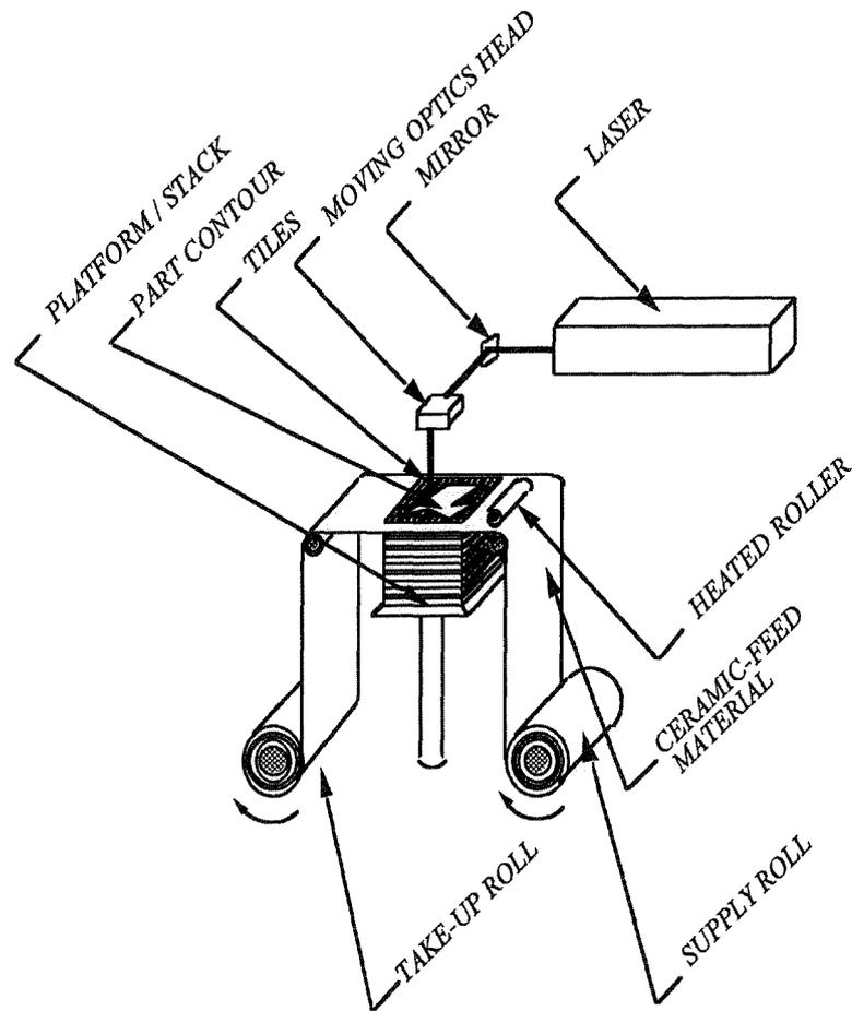
Figure 1. LOM Schematic
