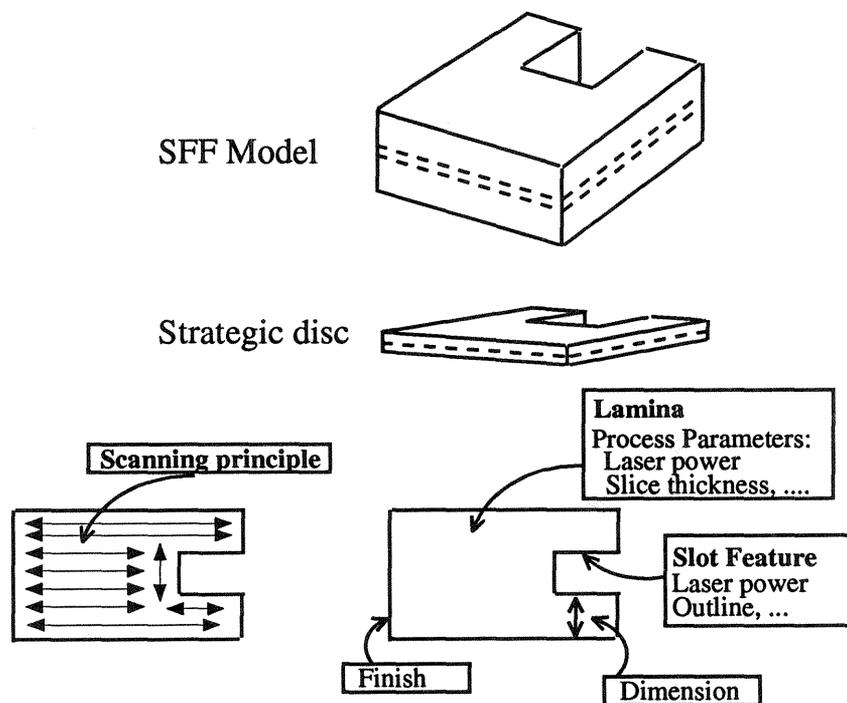
Figure 4 The general SFF model consists of strategic discs accompanied by process parameters and scanning principles.
