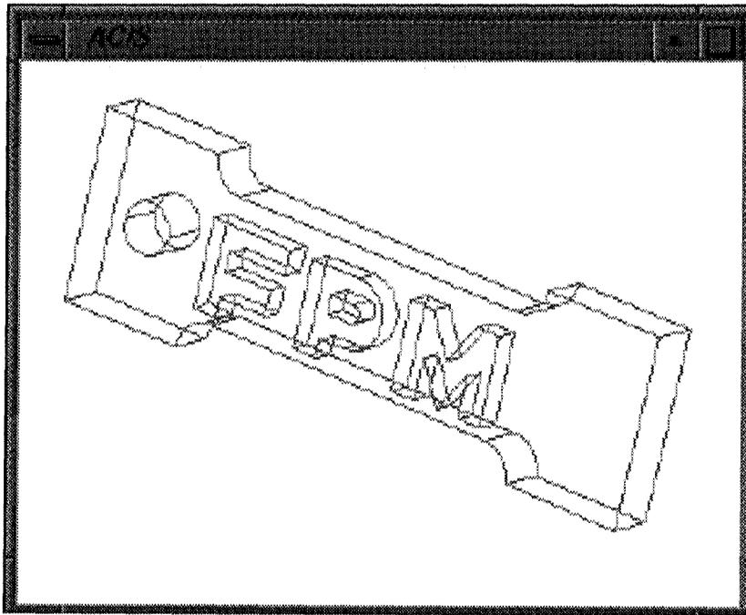
Figure 4 - Key Ring ACIS™ Model Displayed in ACIS Test Harness
