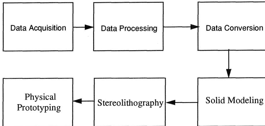
Figure 2: Path from Data Acquisition to Physical Prototype
