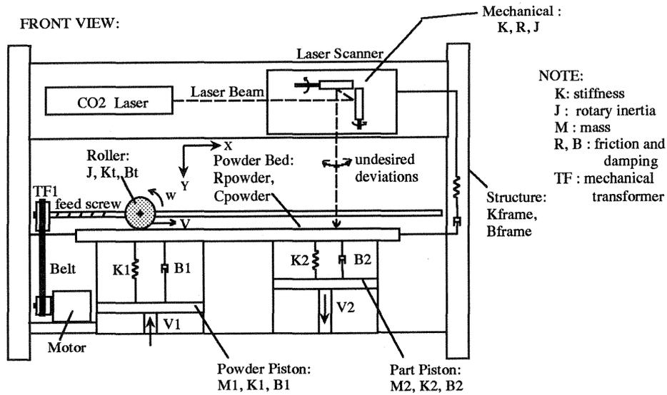
Figure 1: SLS Machine Elements.
