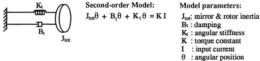
Figure 4: Simple Galvanometer Model.
