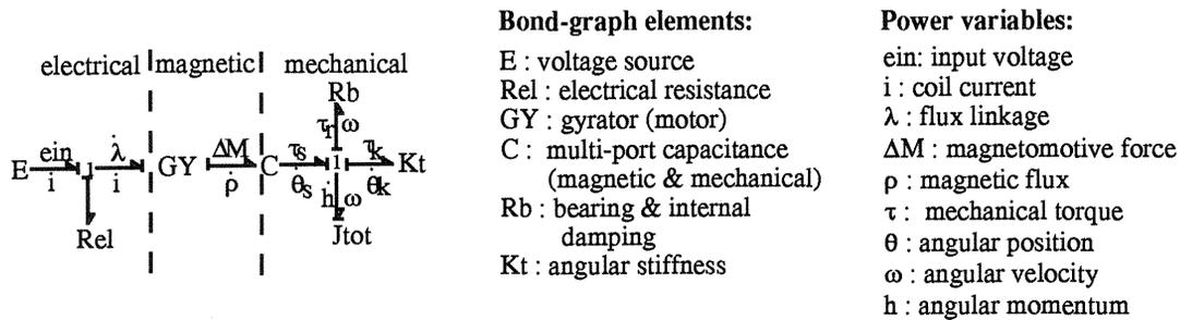
Figure 6: Bond Graph Model of the Galvanometer System.
