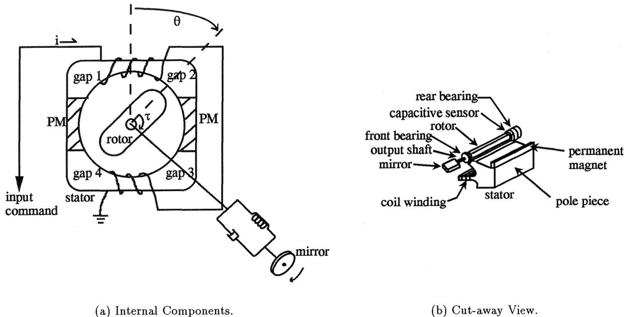
Figure 3: Moving-Iron Galvanometer.
