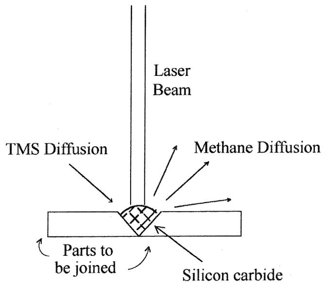
Fig. 2 Detail of deposition area during joining process.
