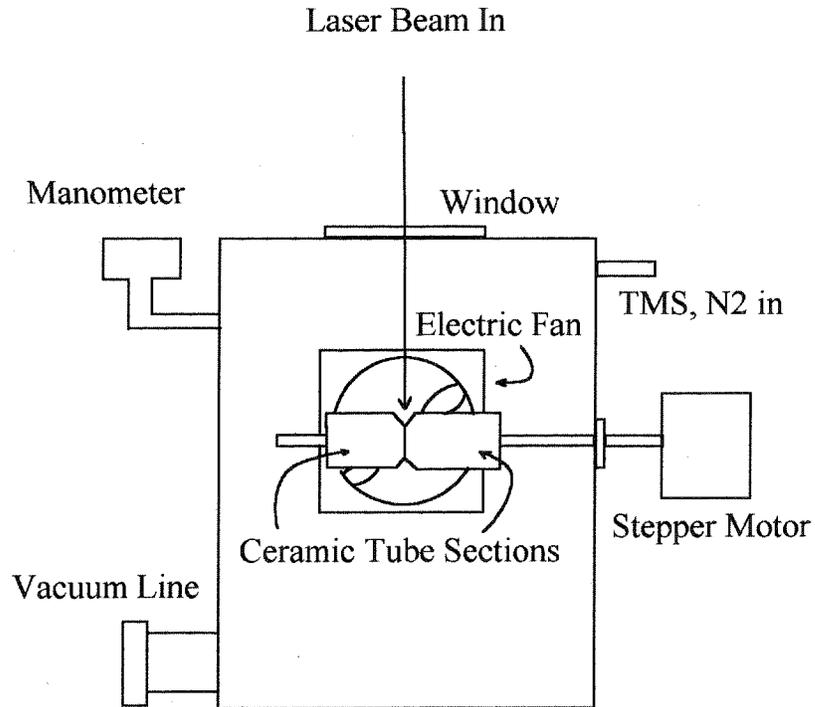
Fig 1. Schematic view of equipment used to evaluate Ceramic Joining by Selected Beam Deposition.
