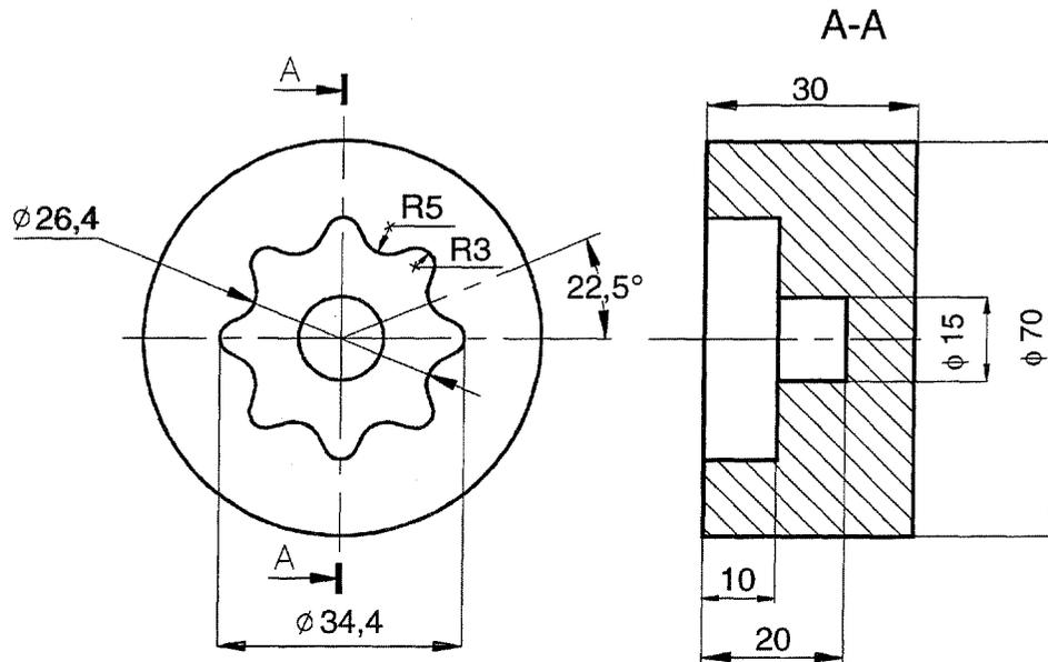
**Figure 1:** Negative master of the EDM electrode.
