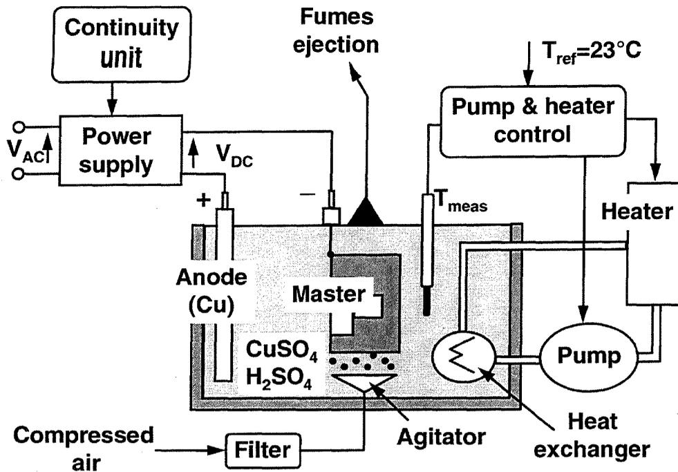
Figure 2: Sketch of the Cu electrodeposition cell.
