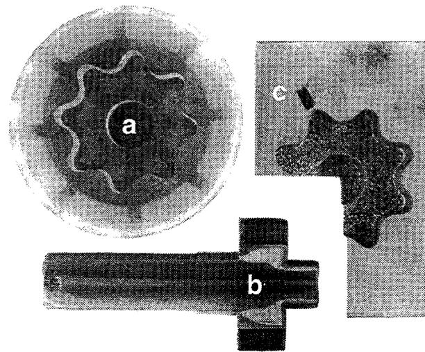
**Figure 3:** a) SLA master, b) Cu electrode, c) workpiece; both electrode and workpiece were sectioned to make SEM observations. On section of electrode is visible the deposited layer of copper.
