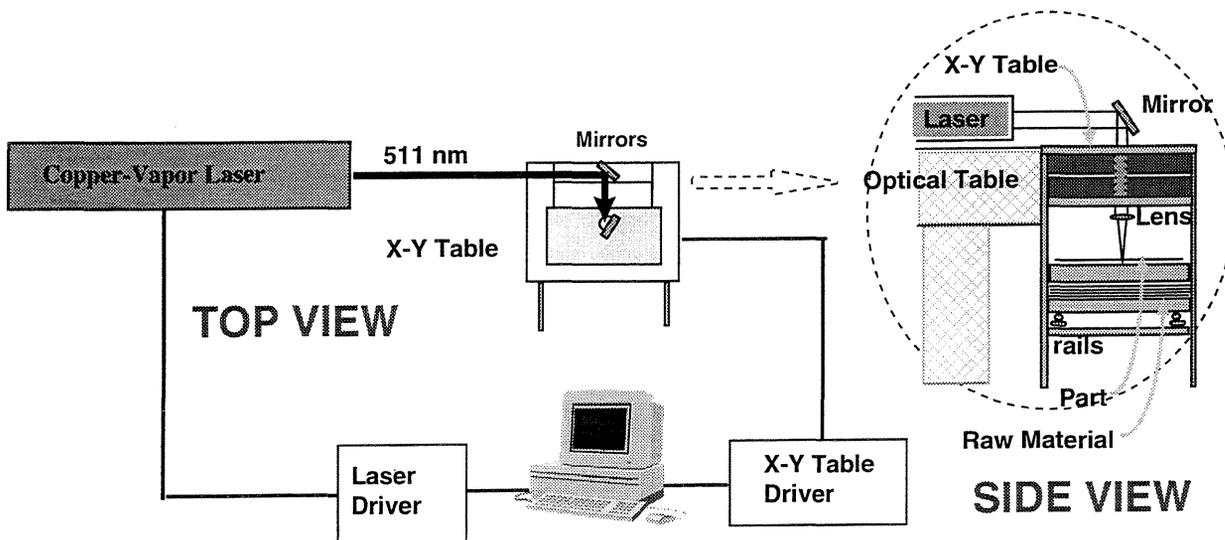
**Figure 1.** Schematic diagram of the TTLOM system.
