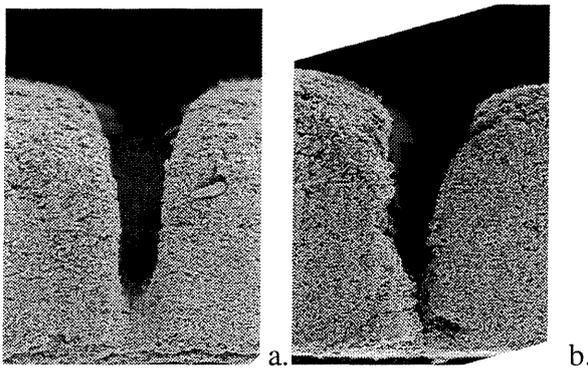
**Figure 4.** Laser cut profiles for different laser operating conditions. (a) Copper-vapor laser -  $1.8\text{mJ}$  per pulse at  $511\text{nm}$  ( $14\text{W}$ ,  $8\text{kpps}$ ,  $20\text{ns}$ , 5 overlap, 7 pass). (b) Nd:YAG tripled -  $25\text{mJ}$  per pulse at  $355\text{nm}$  ( $0.5\text{W}$ ,  $20\text{pps}$ ,  $3\text{ns}$ , 2 overlap, 3 pass).
