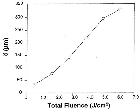
**Figure 7.** Material removal rate (Nicalon fiber) as a function of total fluence deposited for the copper vapor laser. (The line is only a visual guide.)
