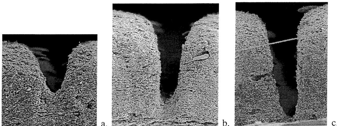
**Figure 6.** Multiple pass material removal, copper-vapor laser and Nicalon tape. (a) 4 passes. (b) 7 passes. (c) 10 passes. Laser kerf is about 80  $\mu$ m.
