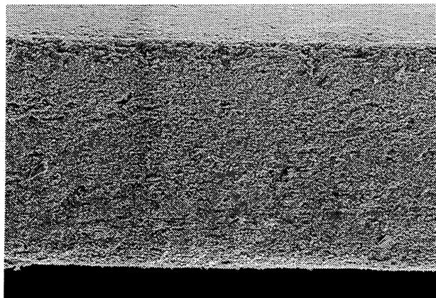
**Figure 5.** Cut edge of Nicalon tape by copper-vapor laser, 1.75mJ per pulse, 5 pulse overlap, 11 passes. Tape is about 350 $\mu$ m thick.
