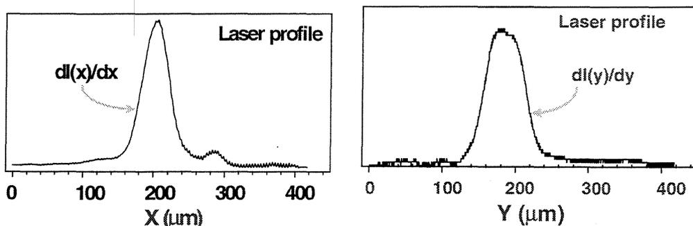
**Figure 2.** Copper-vapor laser profiles at the focal spot.
