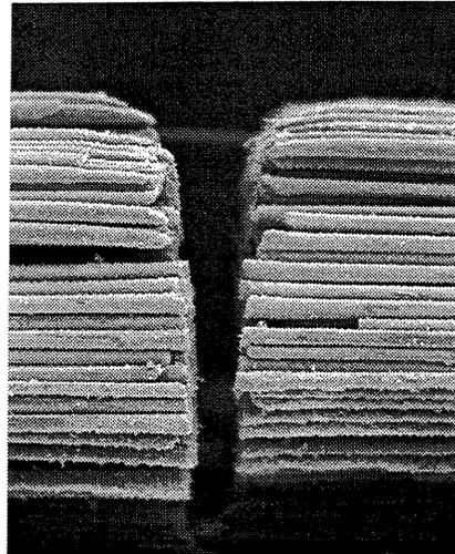
**Figure 8.** Copper-vapor laser penetration of Nicalon fibers. Median kerf is 80 $\mu\text{m}$  and fiber diameter is about 10 $\mu\text{m}$ . (511nm, 14W, 8kpps, 20ns, 5 overlap, 13 pass)
