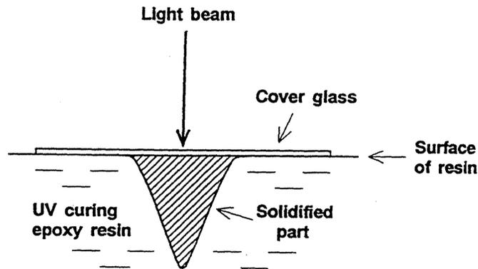
**Fig.4** Illustration of the shape of solidified resin.
