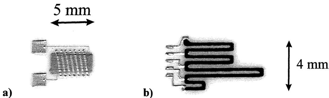
Figure 8. a) Flat solenoid fabricated by connecting lower half windings and upper half windings around thick-film dielectric ( $L(@ 1 \text{ MHz}) \sim 1 \mu\text{H}$ ), b) Multitap voltage divider for 10:1, 7:1, 4:1, and 2:1 voltage division. A  $10\text{k}\Omega/\text{sq}$  resistor with Ag electrodes is used.
