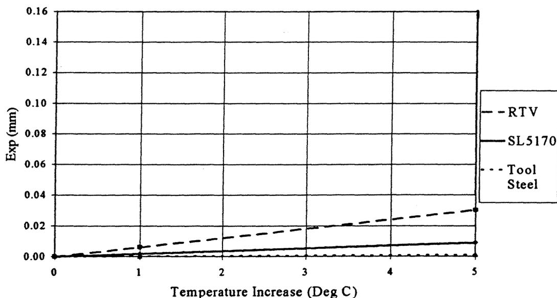
Figure 2: Effect of Increased Temperature on 20mm Dimensions
