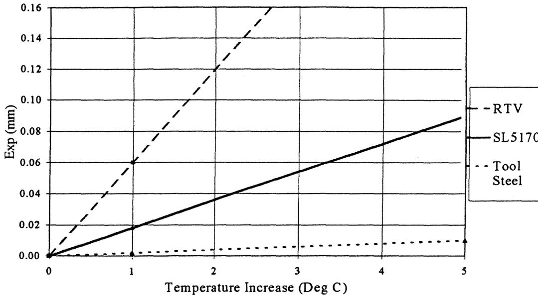
Figure 4: Effect of Increased Temperature on 250mm Dimensions
