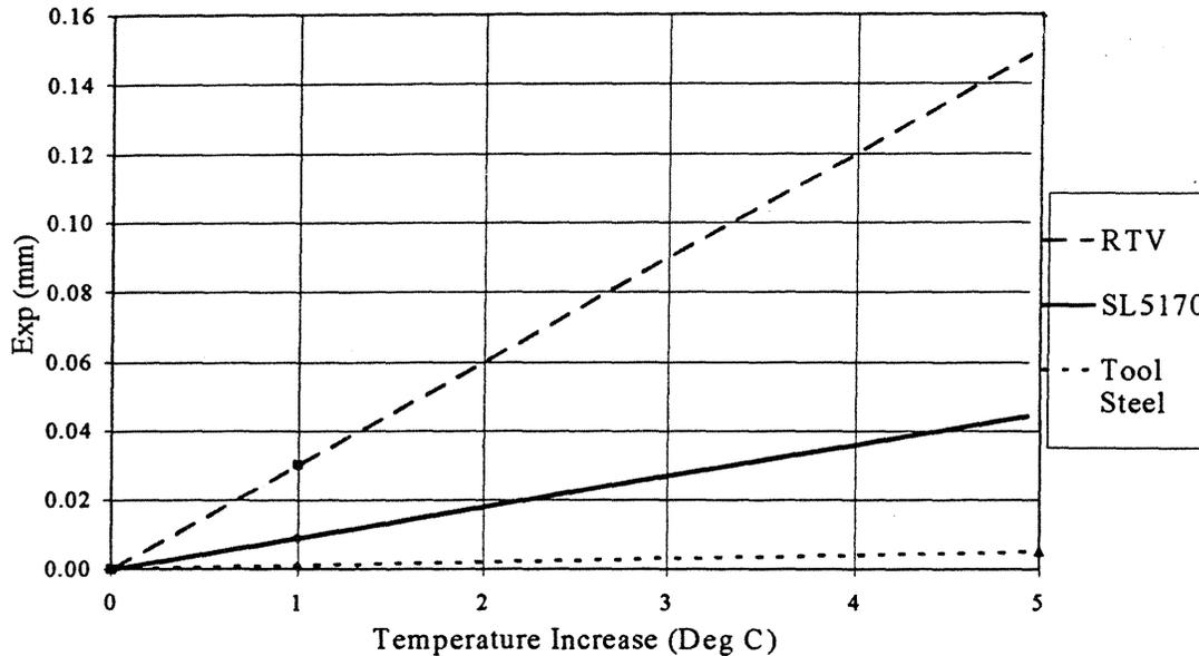
Figure 3: Effect of Increased Temperature on 100mm Dimensions
