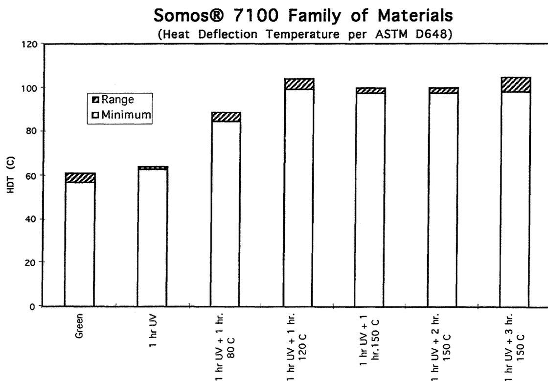
**Figure 1: Heat Deflection Temperature Vs. Thermal Postcure Cycles**
