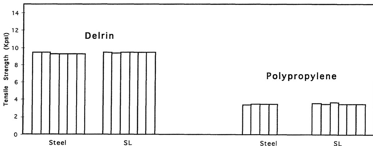
**Figure 4: Strength of the Specimens Molded from Steel and SL Mold Inserts**
