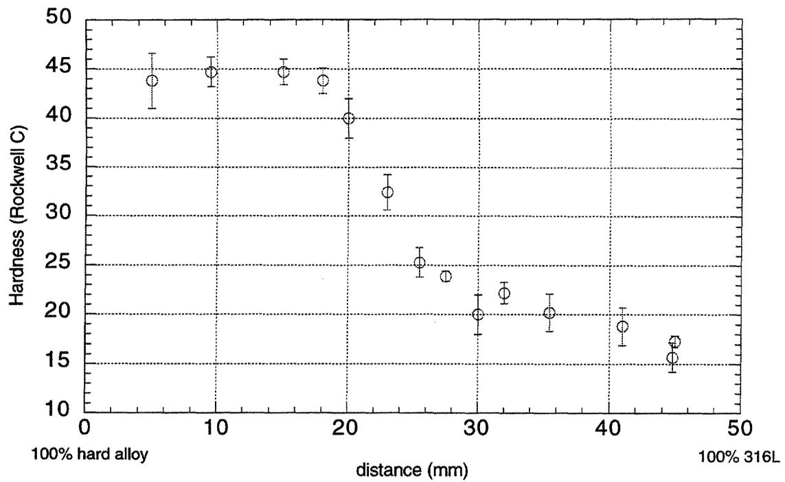
Figure 7: Hardness distribution for a hard alloy to 316L stainless steel graded material.
