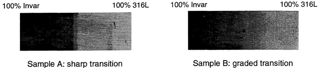
Figure 6: Oxidation of sharp (Sample A) and graded transitions (Sample B) from Invar to stainless steel.
