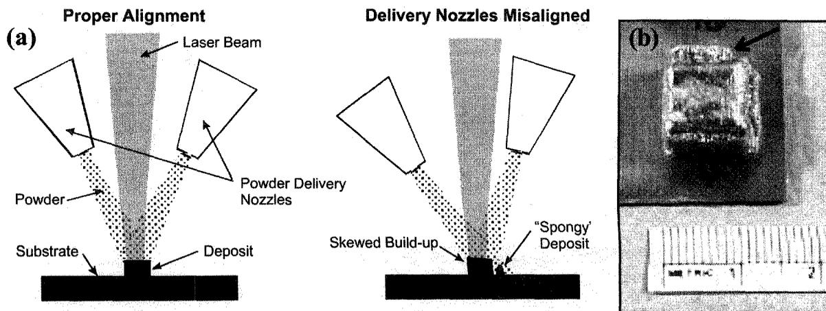
**Figure 3:** (a) Schematic showing how nozzle mis-alignment can affect the quality of the deposit (b) Photo of a sample showing "spongy" deposit on side of cube.
