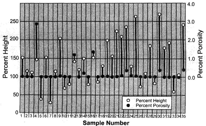
Figure 4: Graph showing the build height and density results for each sample.
