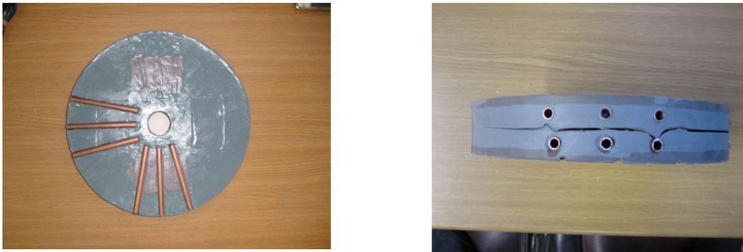
**Fig. 2:** Copper-mixed cavity and cooling pipes in the spin casting mold
