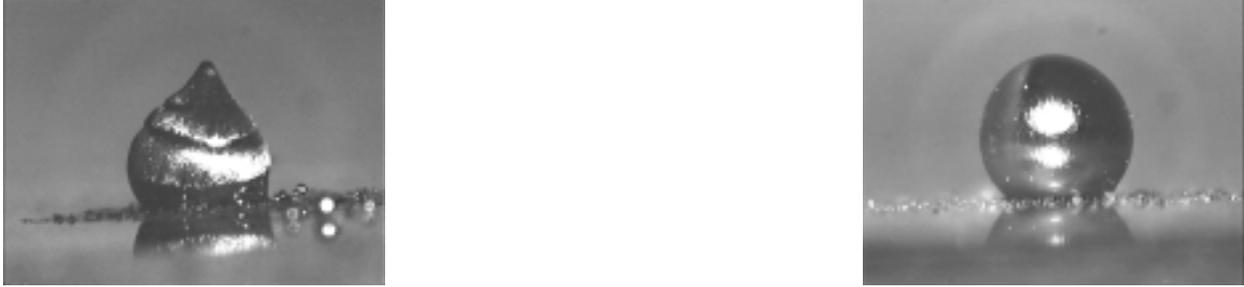
Figure 4: Solidified droplets in “powder on plate” experiment (left) and “strip on plate” experiment (right).
