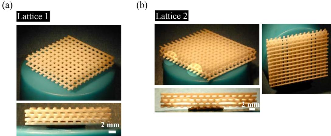
**Figure 2** Aluminum oxide lattices with 8 layers (2 unit cells) having parameters (a)  $d = 2.25$  mm,  $a = 0.64$  mm, filling fraction  $\sim 0.28$  and (b)  $d = 2.3$  mm,  $a = 0.68$  mm, filling fraction  $\sim 0.29$ .
