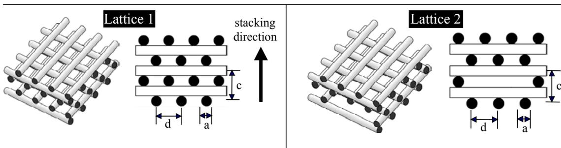
**Figure 1** Schematic illustration of robocasting models where lattice 1 has no missing rods and lattice 2 has a pair of rods removed.
