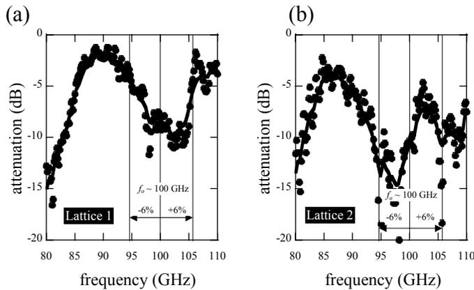
**Figure 3** Attenuation spectra of (a) lattice 1 and (b) lattice 2. The smooth line through the data is simply an aid to guide the eye.
