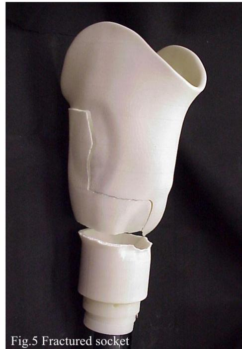
Fig.5 Fractured socket
