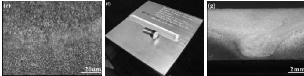
Fig. 3 A laser-deposited H13-steel FSW-tool for the friction-stir welding of aluminum alloys : (a) the as-deposited tool; (b) the tool after hard-turning; (c) cross section of the deposited tool pin; (d) the overlapped laser clad tracks; (e) microstructure at the overlapped region; (f) the tool and the welded 6061 aluminum alloy plate of 6.5 mm in thickness after FSW; (g) cross section of a friction-stir weld of 6061 aluminum to itself.
