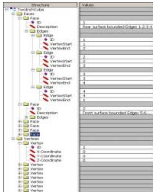
Figure 3b: XML Structure & Data of a 2-inch Cube displayed in XML Notepad
