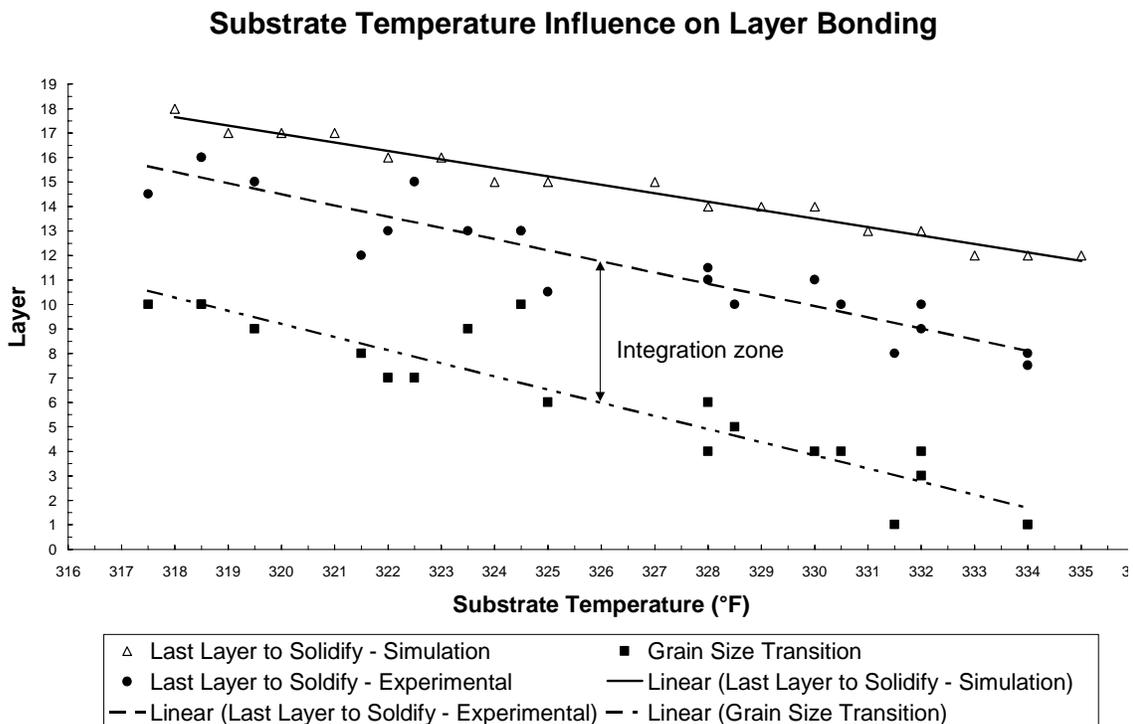
**Figure 8** Comparison of experimental and simulation results
