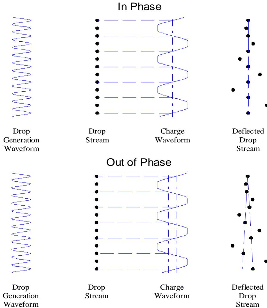
difference between the droplet generation waveform and charge waveform until the center droplets are observed to travel in tandem.
