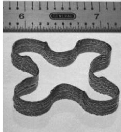
**Figure 1** Thin wall clover built with PDM
