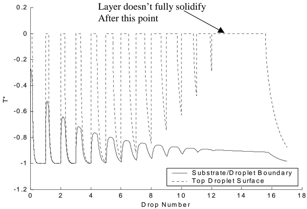
**Figure 7** Simulation of temperature history of the substrate and succession of deposited droplets when substrate is 331 °F.
