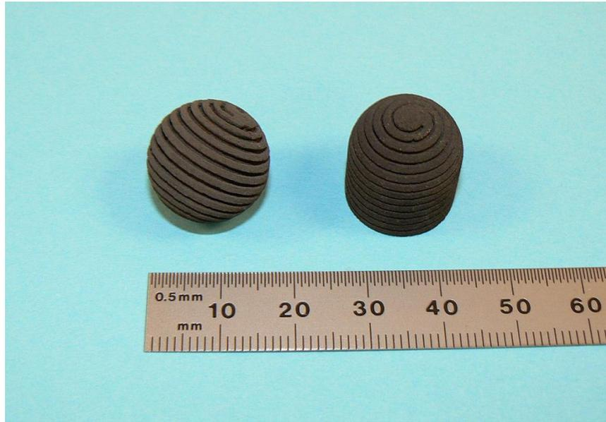
**Figure 4: Printed SS fixtures. The sphere diameter is 17mm, and the hemisphere capped cylinder height and diameter are 17 and 16 mm respectively**
