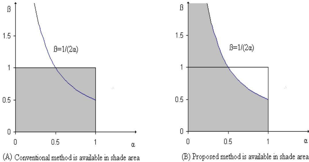
Figure 7: Comparison of applicability of (A) the conventional method and (B) the proposed method for contour measurement of discontinuous surfaces
