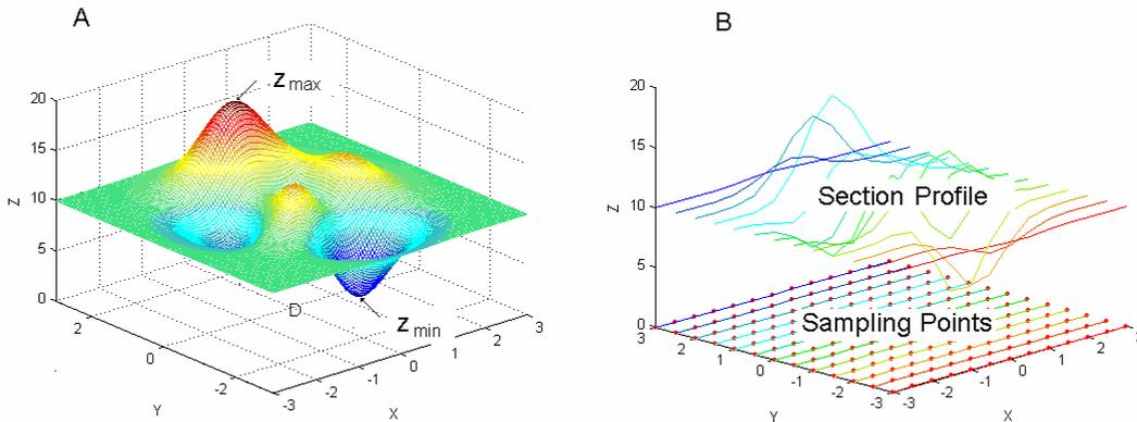
Figure 4: Schematic representation of a component surface for a surface contour measurement
