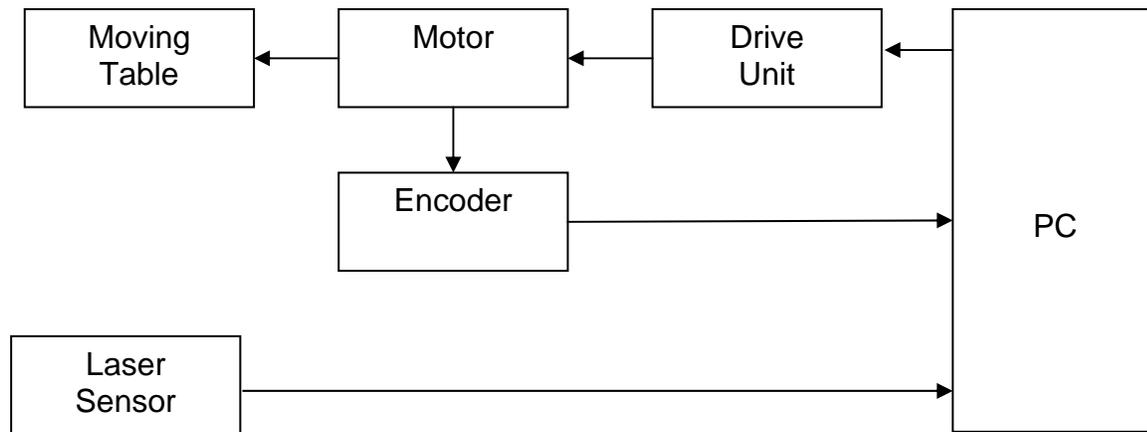
Figure 1: Typical structure of a surface contour measurement system
