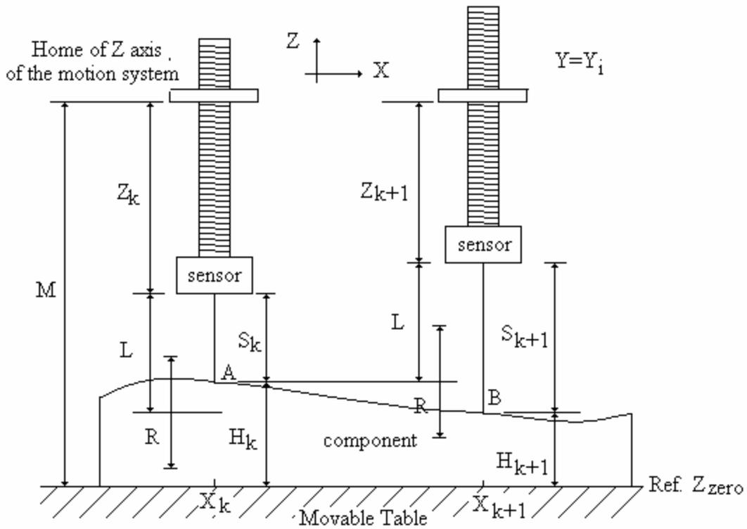
Figure 5: Tracking procedure
