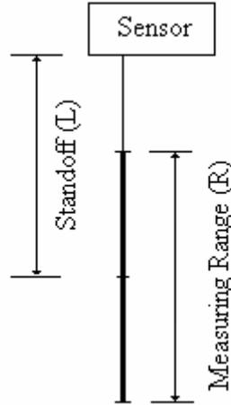
Figure 2: Measurement range and standoff distance of a laser displacement sensor
