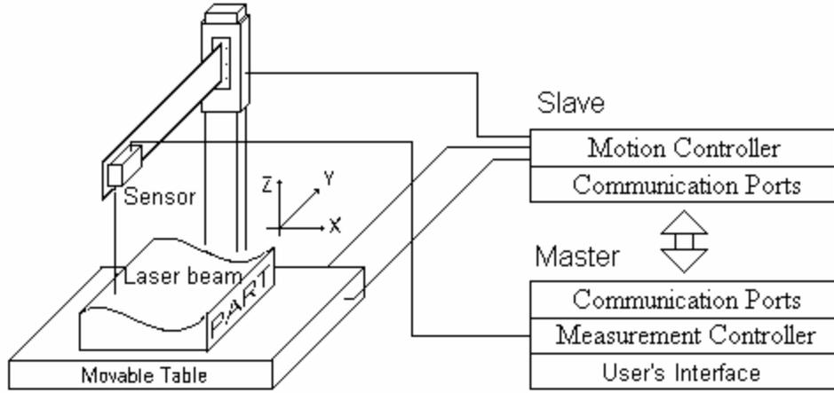
Figure 3: Improved structure of a surface contour measurement system
