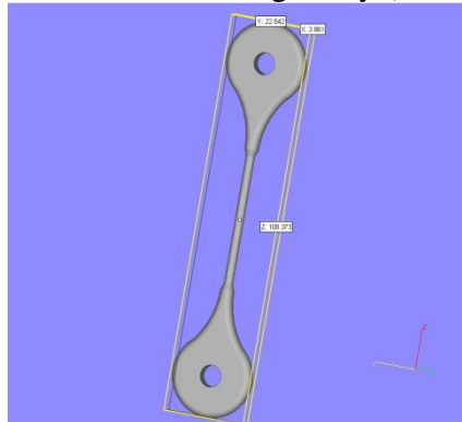
Figure 5: Schematic showing the design of thin round tensile specimens used in case study 2.
