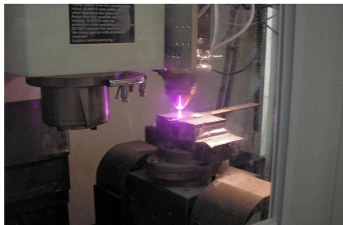
Fig. 1: Laser Aided Manufacturing Process deposition system
