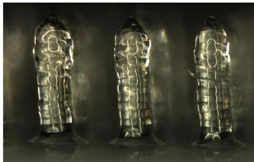
**Figure 12: UV cured silicone posts at 400 um pitch fabricated by dispensing 23 layers of adhesive. Posts measure 175 um in diameter and 800 um tall.**
