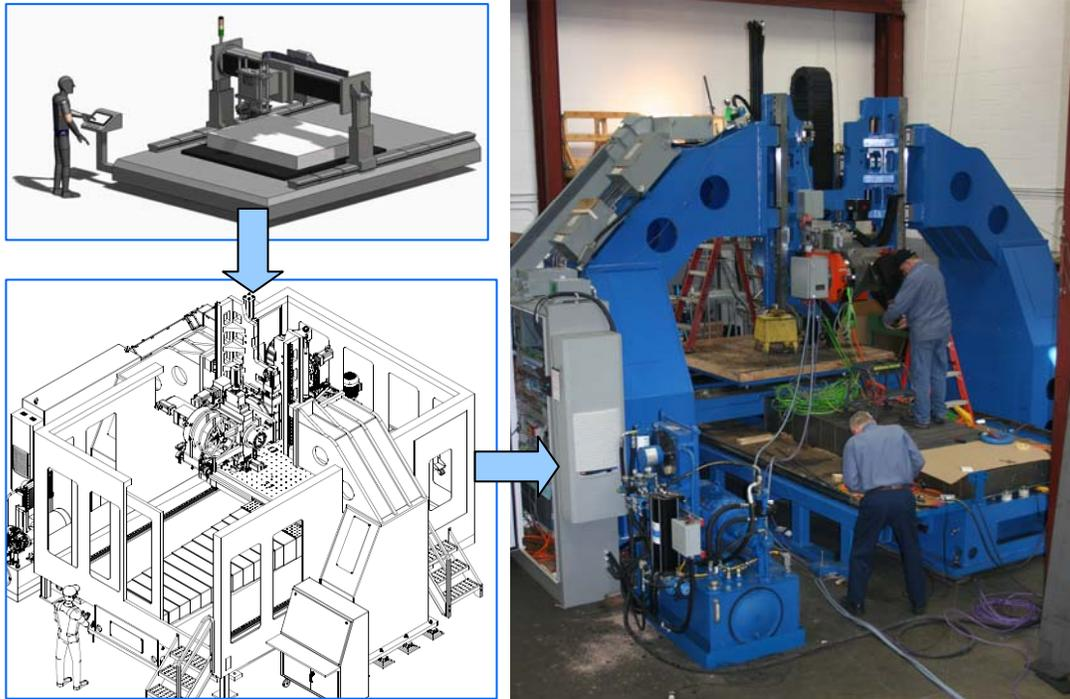
Figure 5. VHP UAM system – from concept to (near) final system
