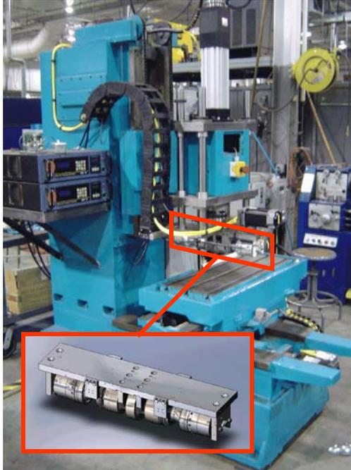
Figure 3. VHP UAM test bed
