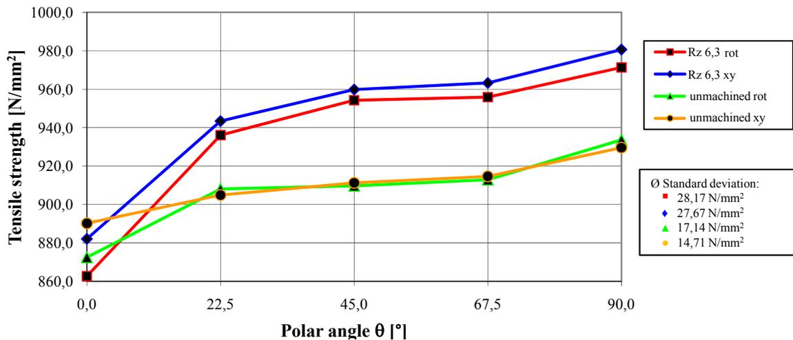
Fig. 5: Tensile strength in dependence on the polar angle  $\theta$  [8]
