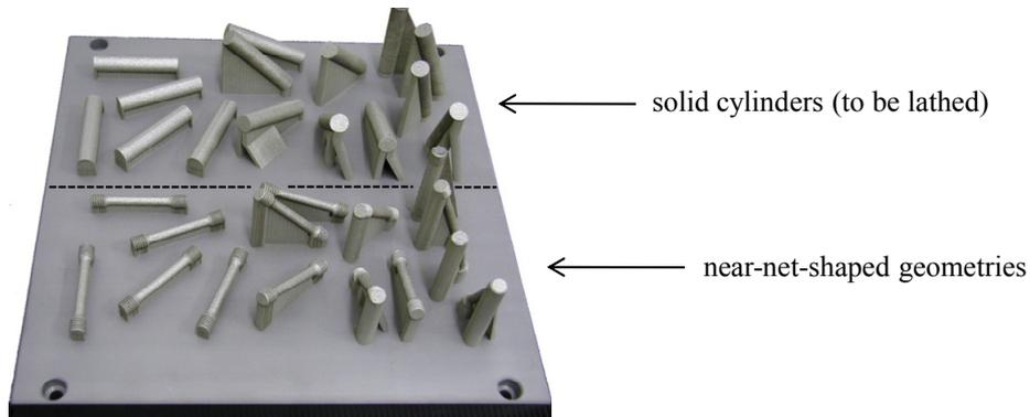
**Fig. 3:** Building platform with two groups of tensile specimens
