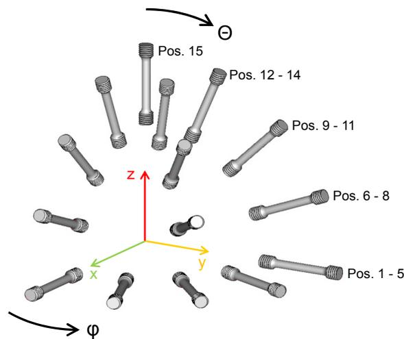
**Fig. 2:** Spatial arrangement of the tensile specimens per group [8]
