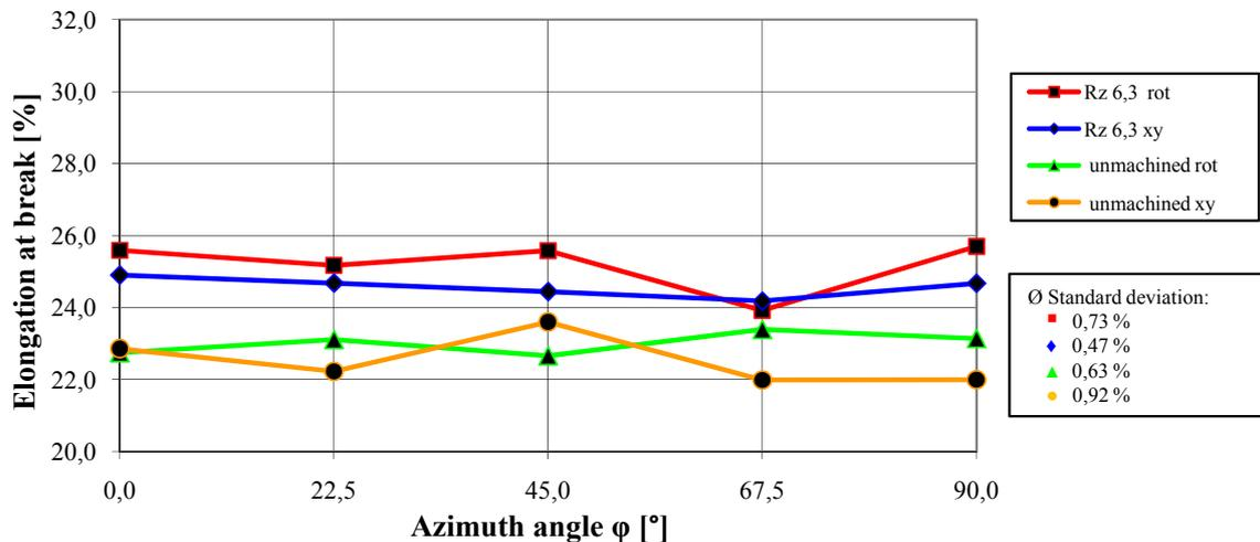
**Fig. 8:** Elongation at break in dependence on the azimuth angle  $\varphi$  [8]
