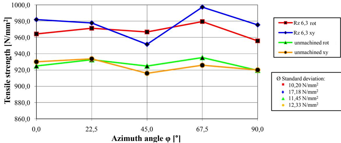
Fig. 6: Tensile strength in dependence on the azimuth angle φ [8]
