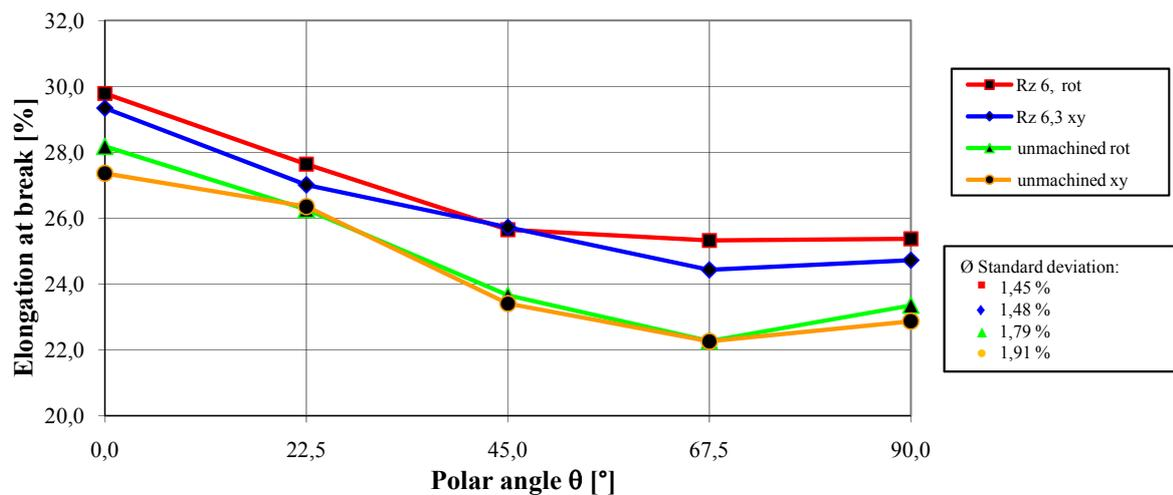
Fig. 7: Elongation at break in dependence on the polar angle θ [8]
