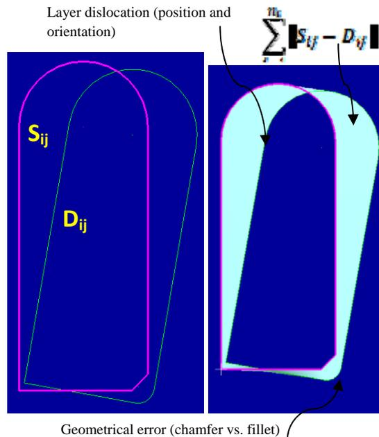
Figure 3. Error calculation for layer k with dislocation and geometrical error.
