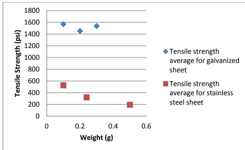
Figure 8. Galvanized and Stainless steel sheet tensile strength comparison based on the bonding mix weight
