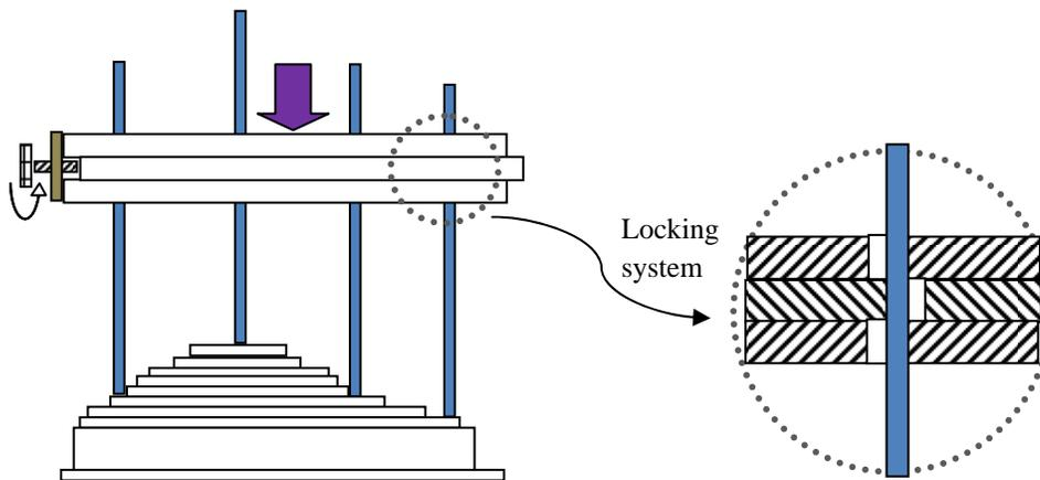
Figure 5. Uniform force distribution to the layers by adjustable pins
