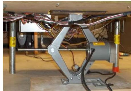
**Compression mechanism.** After all layers are aligned and temporarily bonded, they are placed in the laminating mechanism consists of the compression and heat components. The main requirement for this mechanism is to provide secure clamping on oddly shaped surface, provide sufficient clamping force, provide constant force while heat is applied, and allow for even and thorough application of heat.
