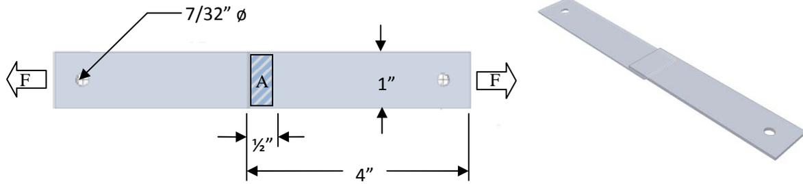
Figure 6. ASTM standard 2294-96 configuration.
