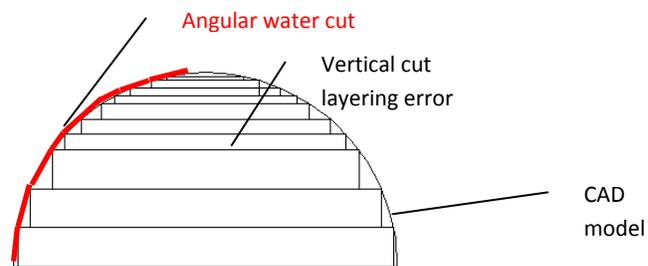
Figure 11. CAD model, layered part, layering error, and near perfect angular abrasive waterjet cutter.
