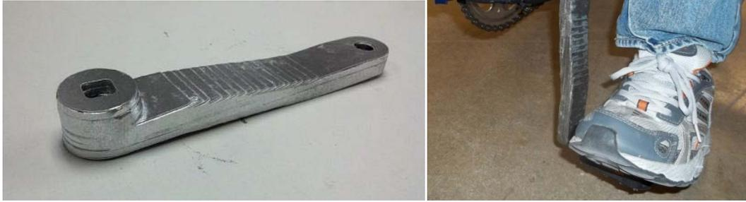
*Figure 10.* Fully dense bike crank manufactured by the FDFE process and functional test
