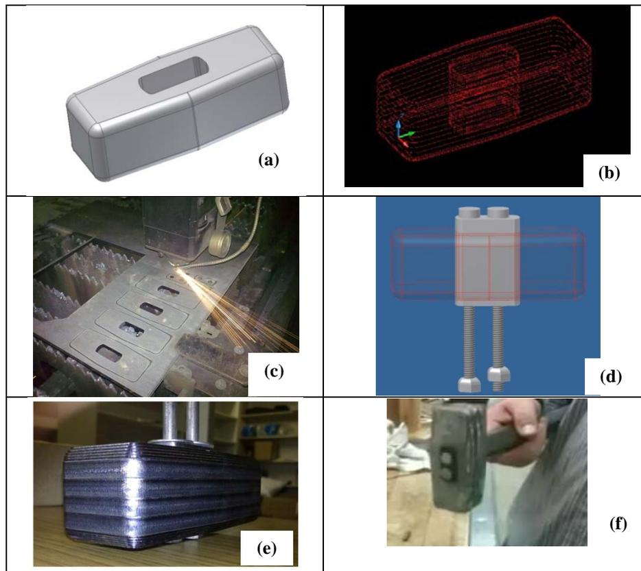
*Figure 1.* General steps for the fully dense freeform fabrication (FDFF) method for a demolition hammer head: 3D solid modeling (a), adaptive slicing (b), abrasive waterjet cutting or laser cutting (c), alignment tooling design (d), bonding layers (e), and final product test (f).
