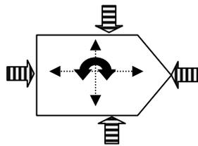
Figure 2. Six movements and four locating points (hatched arrows).
