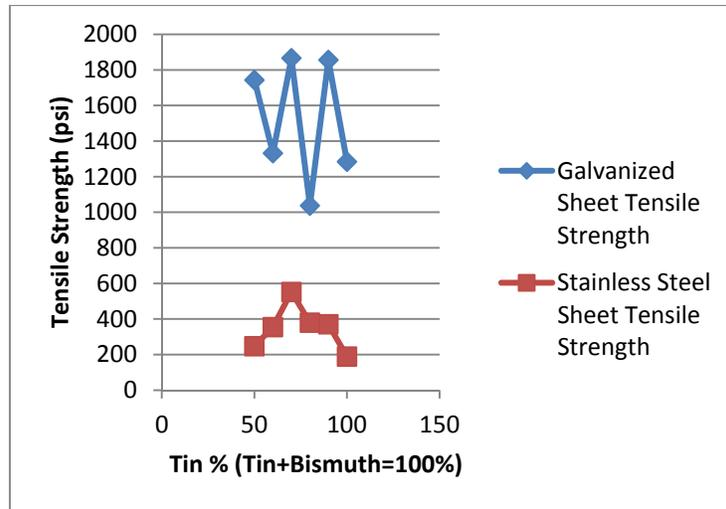
Figure 7. Galvanized and stainless steel sheet tensile strength comparison based on the tin-bismuth percentage
