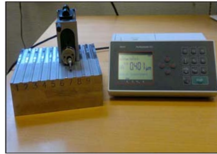
Figure 6: Mahr Perthometer M2 and the milling surface testing sample block.
