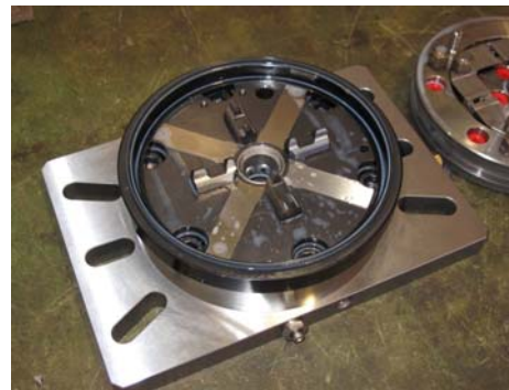
Figure 10: Cutting fluid penetrates the pallet and chuck.
