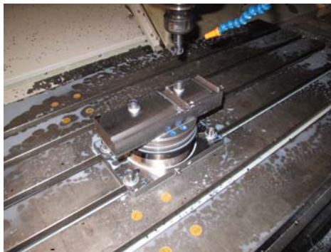
Figure 9: The Erowa PowerChuck and pallet set up for machining test in the Bridgeport VMC
