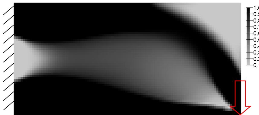
Figure 11: Optimized result for a cantilever plate problem using unpenalized SIMP (i.e. SIM).
