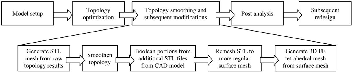
Figure 8: Workflow for topology optimization for AM, with sub-flowchart for the geometry modification stage.
