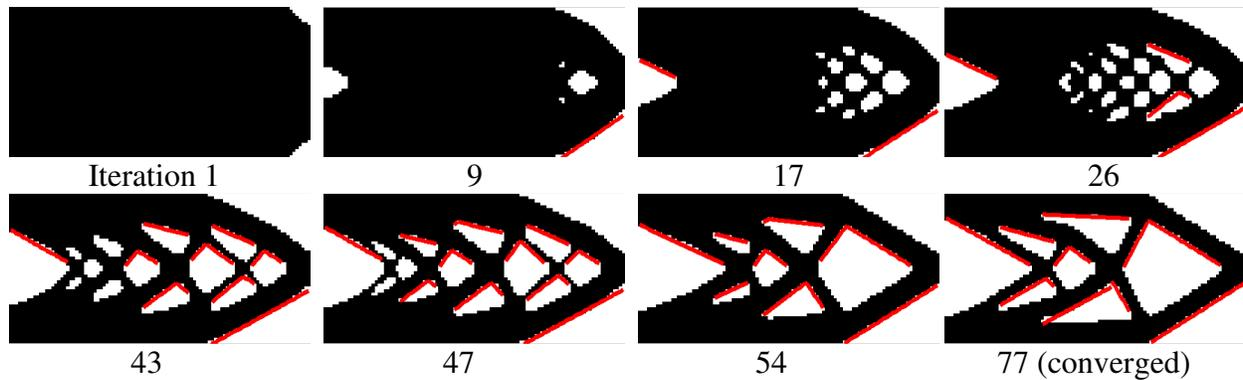
Figure 7 – Iterative downward facing edge analysis during topology optimization, with linear edge approximations plotted in red. Small cavities are ignored due to their inherent self support ability.
