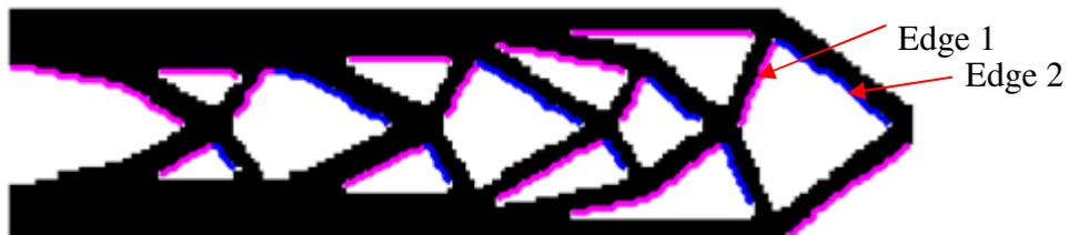
Figure 4: Identification and splitting of the downward facing edges.
