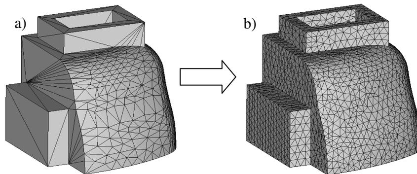
Figure 9: Remeshing an STL to a mesh of better quality for FEA, adapted from [40].
