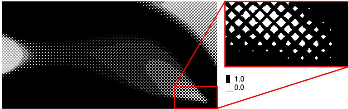
Figure 13: Combined solid and lattice structure by mapping density to unit cells.
