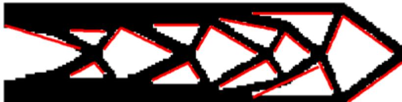
Figure 5: Linear regression fit to the downward facing edge points.
