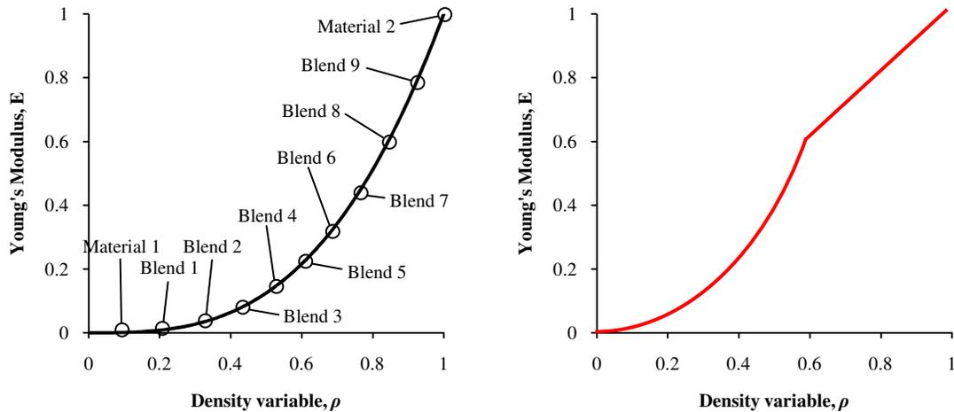
Figure 14: a) SIMP material interpolation scheme with penalization,  $p = 3$ , with example corresponding jetted materials/blends, and b) Potential interpolation scheme to include manufacturable functional density variation above 60%.
