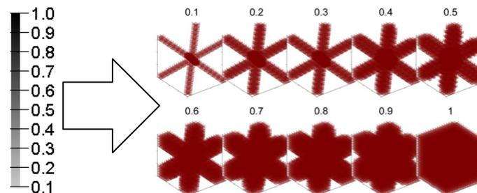
Figure 12: Mapping of variable density to variable volume fraction lattice unit cells.
