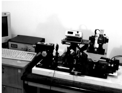
Fig.12 Laser-guided direct transportation system
