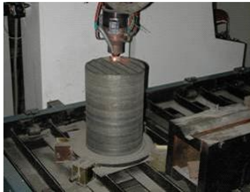
Fig. 10 AM process based on high-energy laser beams
