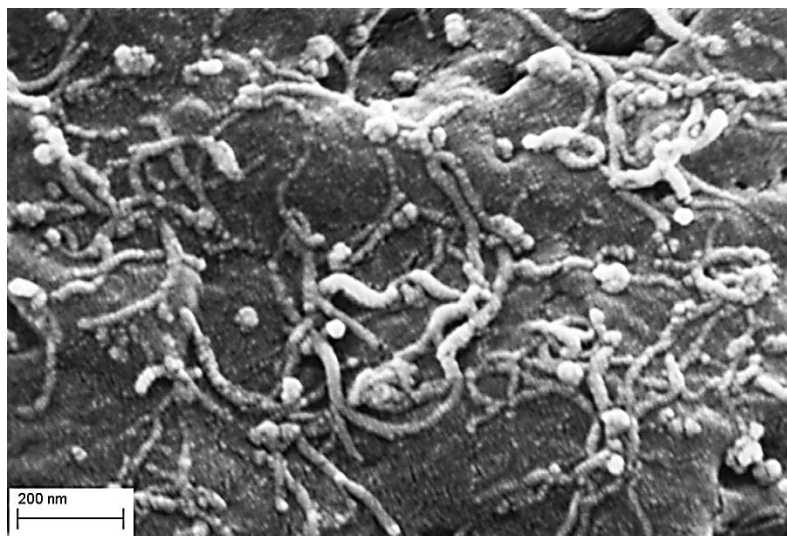
Figure 4: SEM micrograph of CNT (white strands) dispersion in the PA12 matrix
