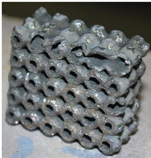
**Figure 10. Successful complex, hollow, metal geometry made with SLS, ENP and flash burnout (27mm wide).**
