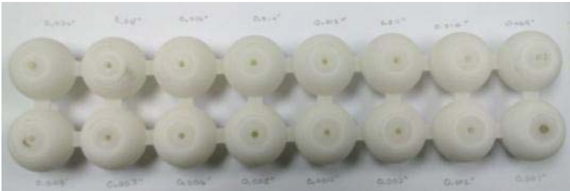
Figure 13: Fused spherical joints with varying tolerances.
