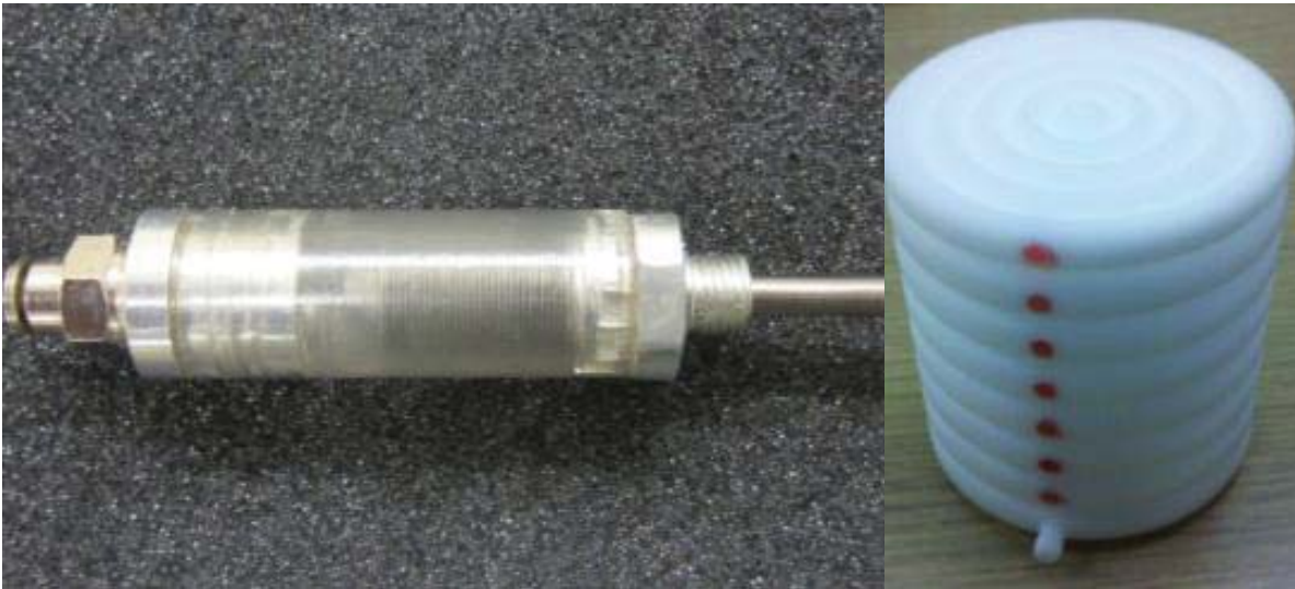
Figure 3: Bellows actuators designed and manufactured at MSOE.
