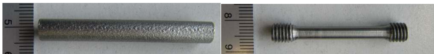
Figure 1: Tensile specimens (190W, 800mm/s) – horizontally produced blank (left) and final drilled specimen according to DIN-50125-form B (right).
