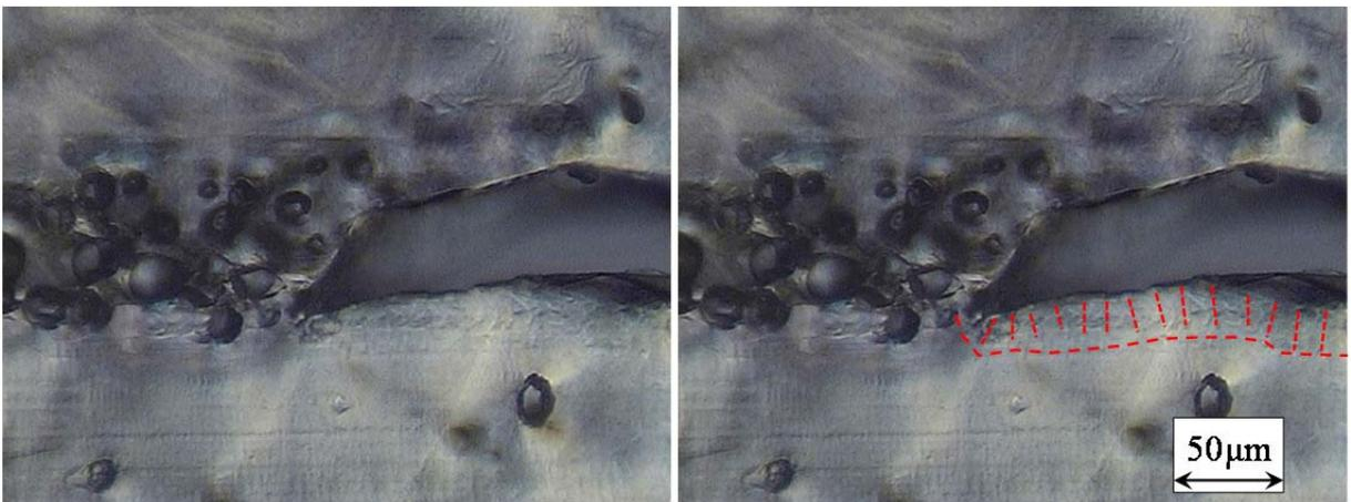
**Figure 8** Polarized optical transmission micrograph of a PF processed part. Striped contrasts are found near the pore edge as shown in the right picture.
