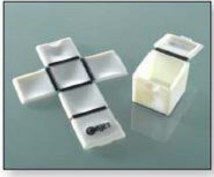
Figure 2: A 3DP part with elastomer living hinges (shown in black) [1]
