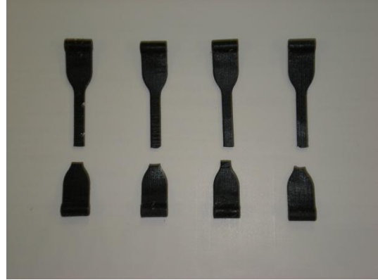
Figure 7: Pictures of the breaks at the TangoBlackPlus specimen neck
