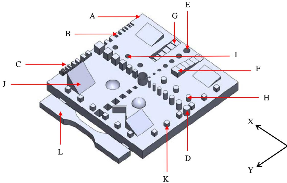
Figure 1. Design of test part used for the ranking model and the orientation in which the part was built
