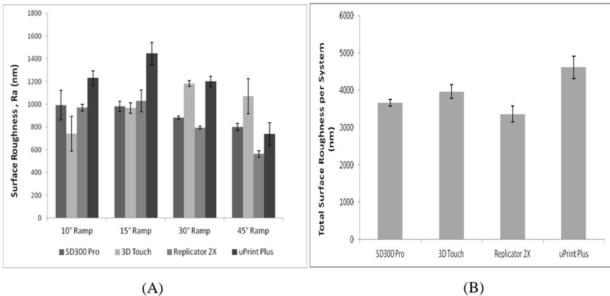
Figure 4. (A) Surface roughness with respect to various angles; (B) Total surface roughness per system
