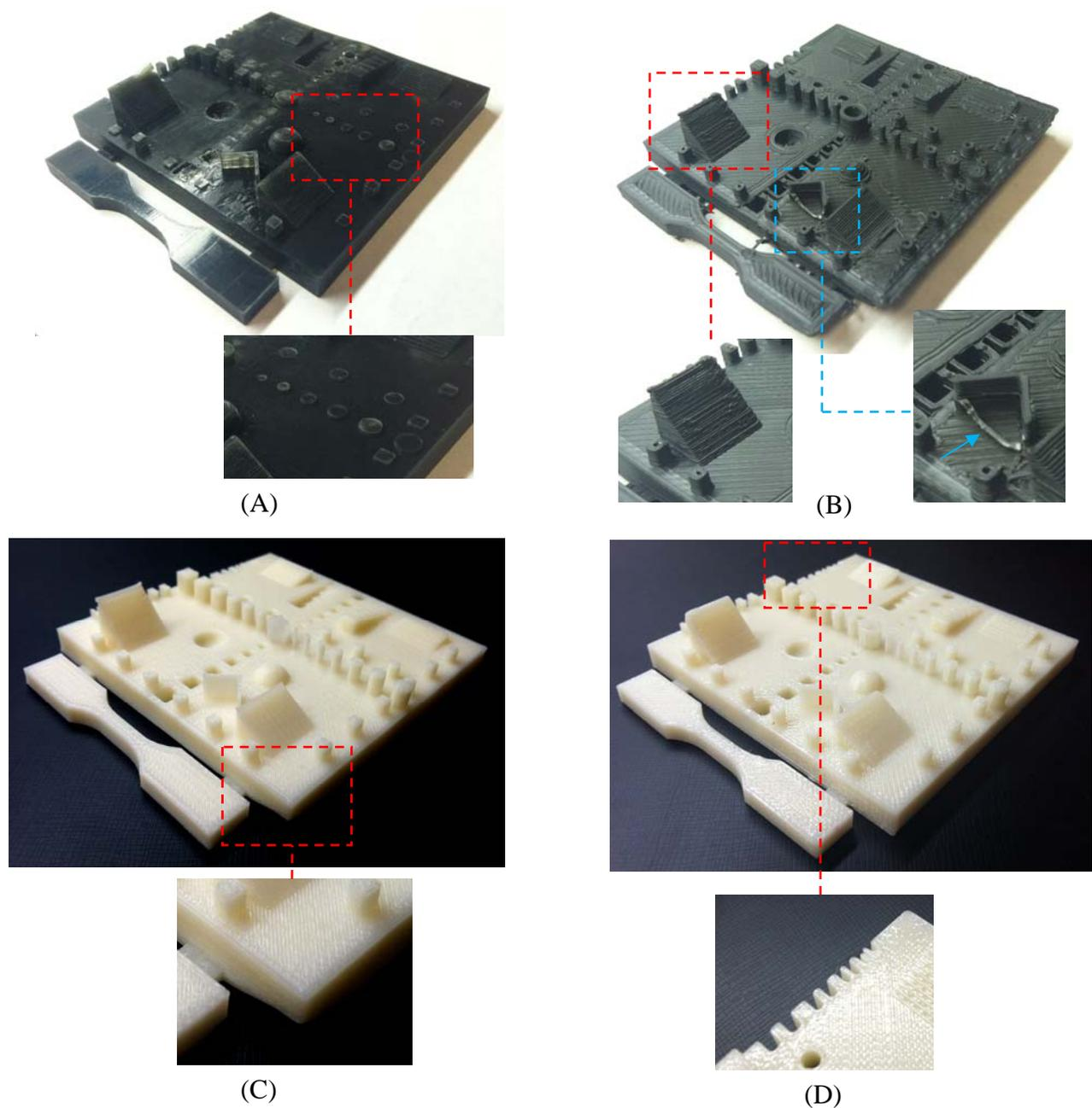
Figure 3. Test part built with the four systems: (A) SD300 Pro; (B) 3D Touch; (C) Replicator 2X; (D) uPrint Plus
