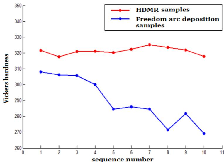
Figure 3 Hardness distributions between freedom arc deposition samples and HDMR samples
