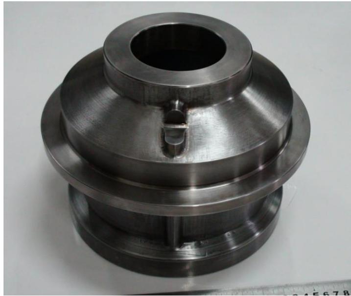
Figure 5 a 45 steel aeronautical part manufactured by the HDMR method (after milling)
