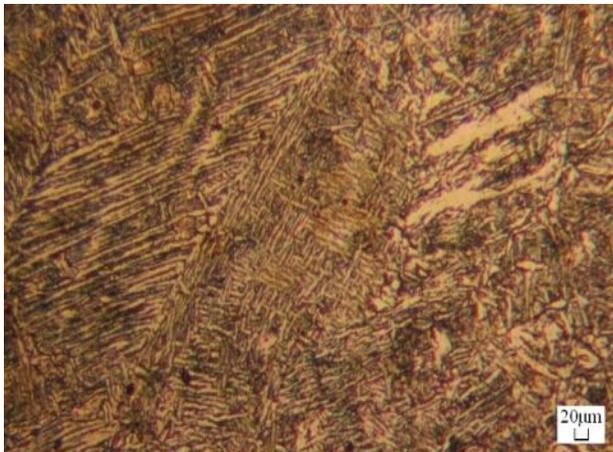
(c) Freedom arc deposition metallographic phase
