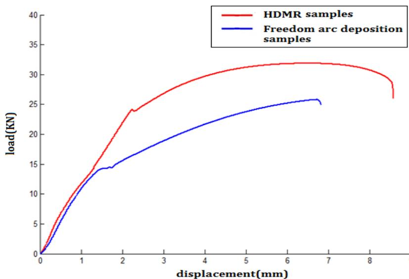
Figure 4 Tensile displacement-load curves between freedom arc deposition process and HDMR process
