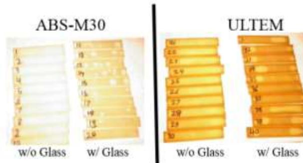
Figure 6 – Specimens fabricated for the second experiment, internal voids are visible.
