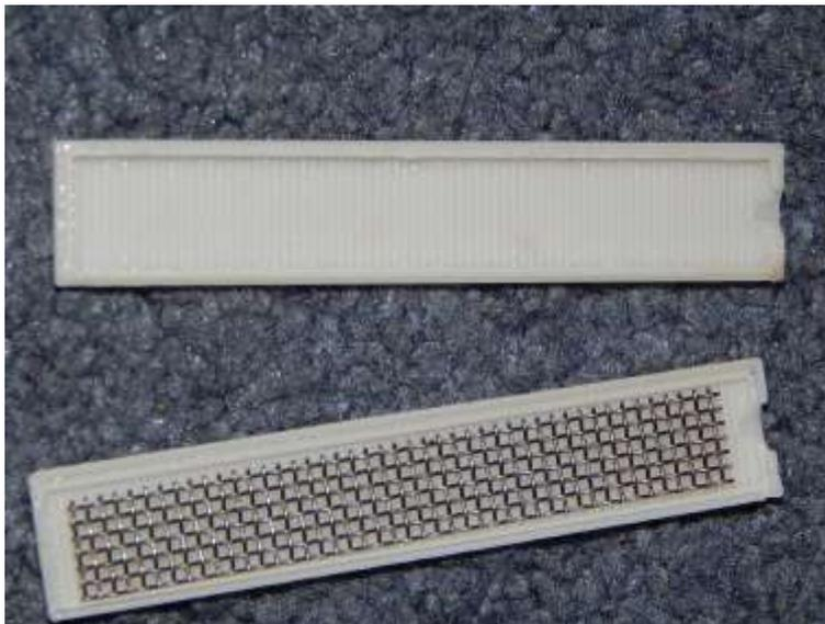
Figure 2 - Interlocking 3D printed thin skins showing the opening on the right side for injecting the adhesive by syringe.
