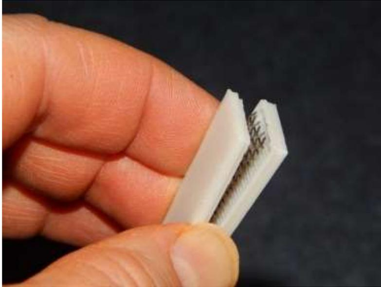
Figure 1 - Interlocking 3D printed thin skins with stainless steel mesh inside.
