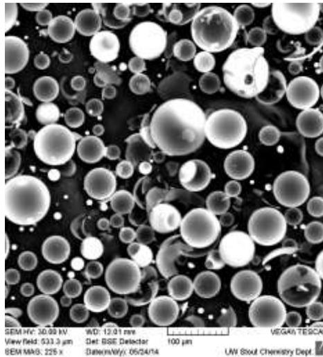
Figure 7 – Image shows the size distribution of the glass microspheres.
