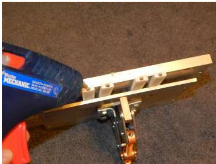
Figure 3 - Specimens being prepared by injecting the adhesive in the first experiment.
