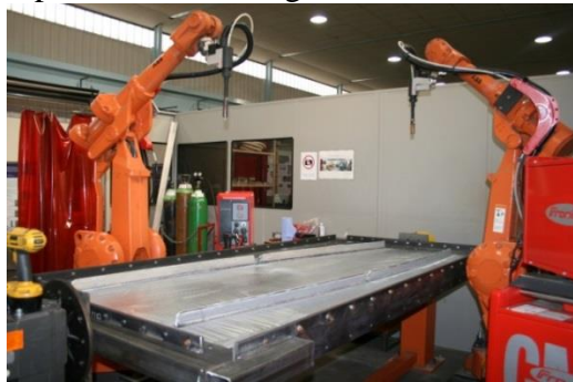
Figure 11 Multiple robots building a long Aluminum rib
