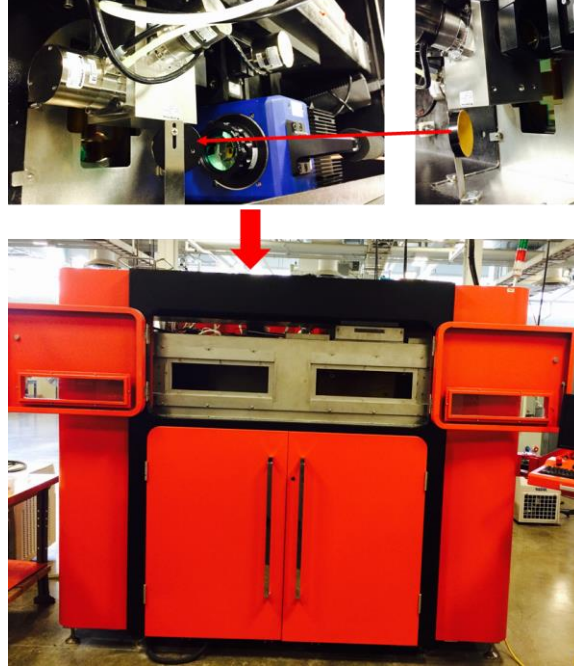
Figure 2. System setup consists of the new “open architecture” LS machine, thermal camera and a 2 in flat gold mirror.
