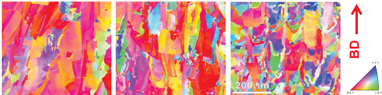
Figure 6 IPF maps for Haynes® 230® using (a) 116 J/mm 3 , (b) 77 J/mm 3 and (c) 66 J/mm 3 (directly adapted from Bauer et al. [24])
