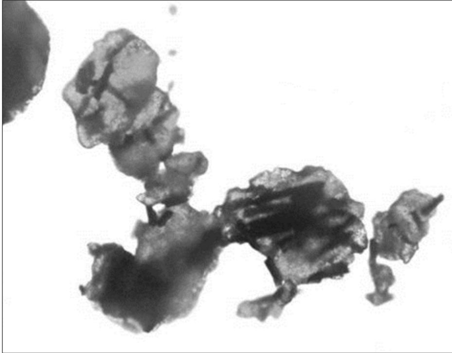
Figure 2: Micrograph of HT23 powder grains with encapsulated carbon fibers.
