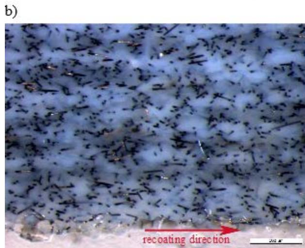
Figure 3: Micrographs of part cross sections. a) Cuts in three directions through a cuboid laser part made from HT23. b) Cross section of a laser sintered part made from a HP3/carbon fiber dry-blend. The recoating direction is indicated in red.
