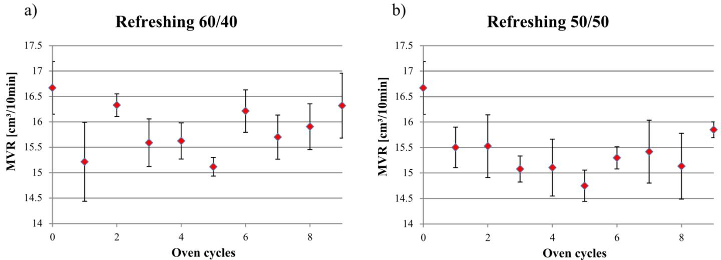
Figure 4: Simulation of 9 cycles of building and refreshing the powder. Cycle "0" indicates the melt volume rate (MVR) of new powder. After every cycle, the powder was blended with 60% (a) or 50% (b) new powder and aged again.
